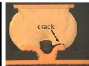
Figure 14. Cracks in a Micro-via Void-containing corner solder joint of a BGA package (Left) and no crack in the adjacent solder joint (Right), which contains a Micro-via Void.
