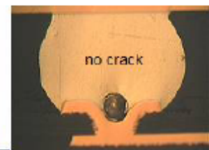
Figure 14. Cracks in a Micro-via Void-containing corner solder joint of a BGA package (Left) and no crack in the adjacent solder joint (Right), which contains a Micro-via Void.
